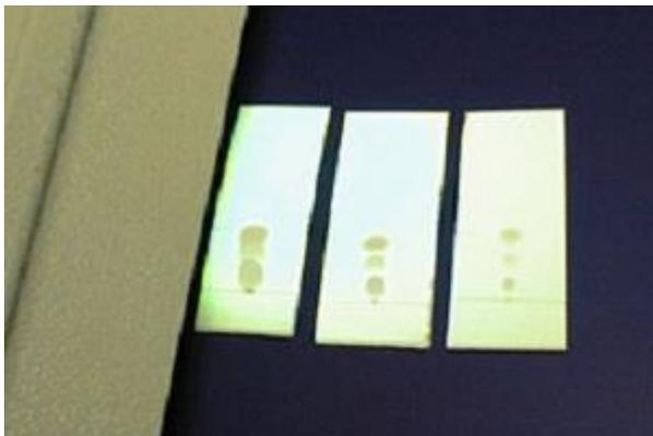
If the TLC plate runs samples which are too concentrated, the spots will be streaked and/or run together. If this happens, you will have to start over with a more dilute sample to spot and run on a TLC plate.
