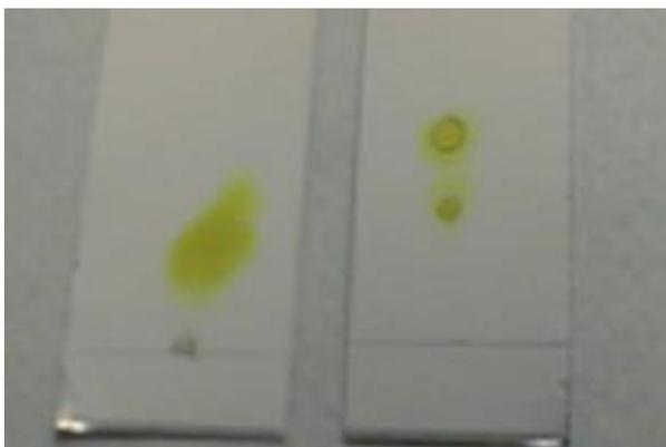
Here's what overloaded plates look like compared to well-spotted plates. The plate on the left has a large yellow smear; this smear contains the same two compounds which are nicely resolved on the plate next to it.
