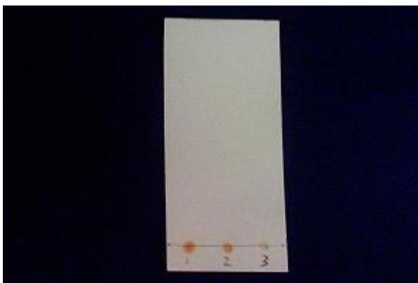
This example plate has been spotted with three different quantities of the same solution and is ready to develop. If you are unsure of how much sample to spot, you can always spot multiple quantities and see which looks best.
