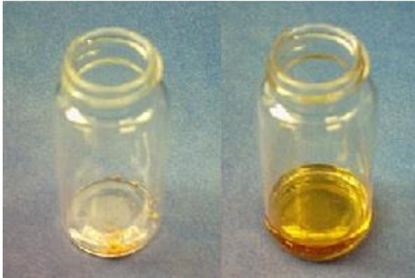
If the sample is not already in solution, dissolve about 1 mg in 1 mL of a volatile solvent such as hexanes, ethyl acetate, or methylene chloride. As a rule of thumb, a concentration of 1% usually works well for TLC analysis. If the sample is too concentrated, it will run as a smear or streak (see troubleshooting section below); if it is not concentrated enough, you will see nothing on the plate. Sometimes you will need to use trial and error to get well-sized, easy to read spots.
