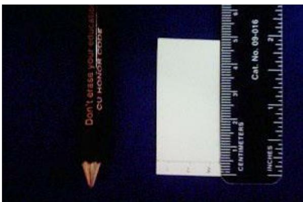
Measure 0.5 cm from the bottom of the plate. Using a pencil, draw a line across the plate at the 0.5 cm mark. This is the *origin*: the line on which you will spot the plate. Take care not to press so hard with the pencil that you disturb the adsorbent. Under the line, mark lightly the name of the samples you will spot on the plate, or mark numbers for time points. Leave enough space between the samples so that they do not run together; about 4 samples on a 5 cm wide plate is advised.
