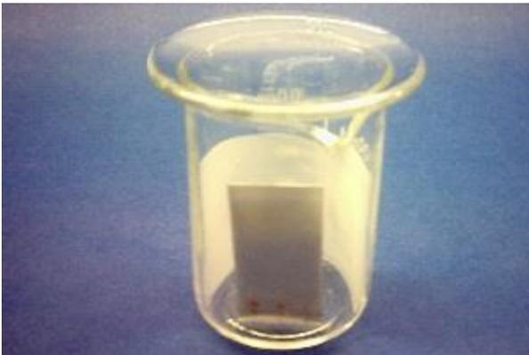
Allow the plate to develop until the solvent is about half a centimeter below the top of the plate. Remove the plate from the beaker and immediately mark the solvent front with a pencil. Allow the plate to dry.
