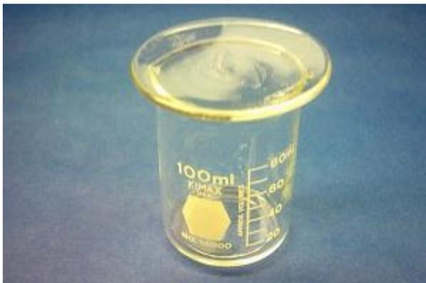
The developing container for TLC can be a specially designed chamber, a jar with a lid, or a beaker with a watch glass on the top (the latter is used in the undergrad labs at CU). Pour solvent into the chamber to a depth of just less than 0.5 cm. To aid in the saturation of the TLC chamber with solvent vapors, you can line part of the inside of the beaker with filter paper. Cover the beaker with a watch glass, swirl it gently, and allow it to stand while you prepare your TLC plate.
