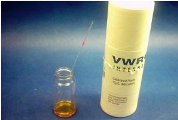
Obtain a microcapillary. In the organic teaching labs, we use 10 $\mu$ L microcaps - they are easier to handle than the smaller ones used in research labs. Dip the microcap into the solution and then **gently** touch the end of it onto the proper location on the TLC plate. Don't allow the spot to become too large - if necessary, you can touch it to the plate, lift it off and blow on the spot. If you repeat these steps, the wet area on the plate will stay small.
