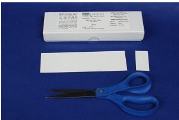
TLC plates used in the organic chem teaching labs are purchased as 5 cm x 20 cm sheets. Each large sheet is cut horizontally into plates which are 5 cm tall by various widths; the more samples you plan to run on a plate, the wider it needs to be. Shown in the photo to the left is a box of TLC plates, a large un-cut TLC sheet, and a small TLC plate which has been cut to a convenient size. Handle the plates carefully so that you do not disturb the coating of adsorbent or get them dirty.
