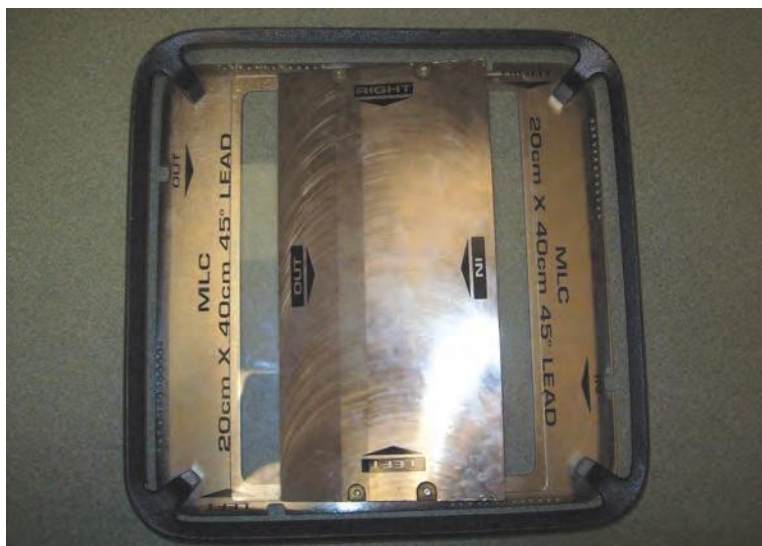
Figure 11.7. Photograph of a 45-degree wedge filter (Varian 21 EX linac).
