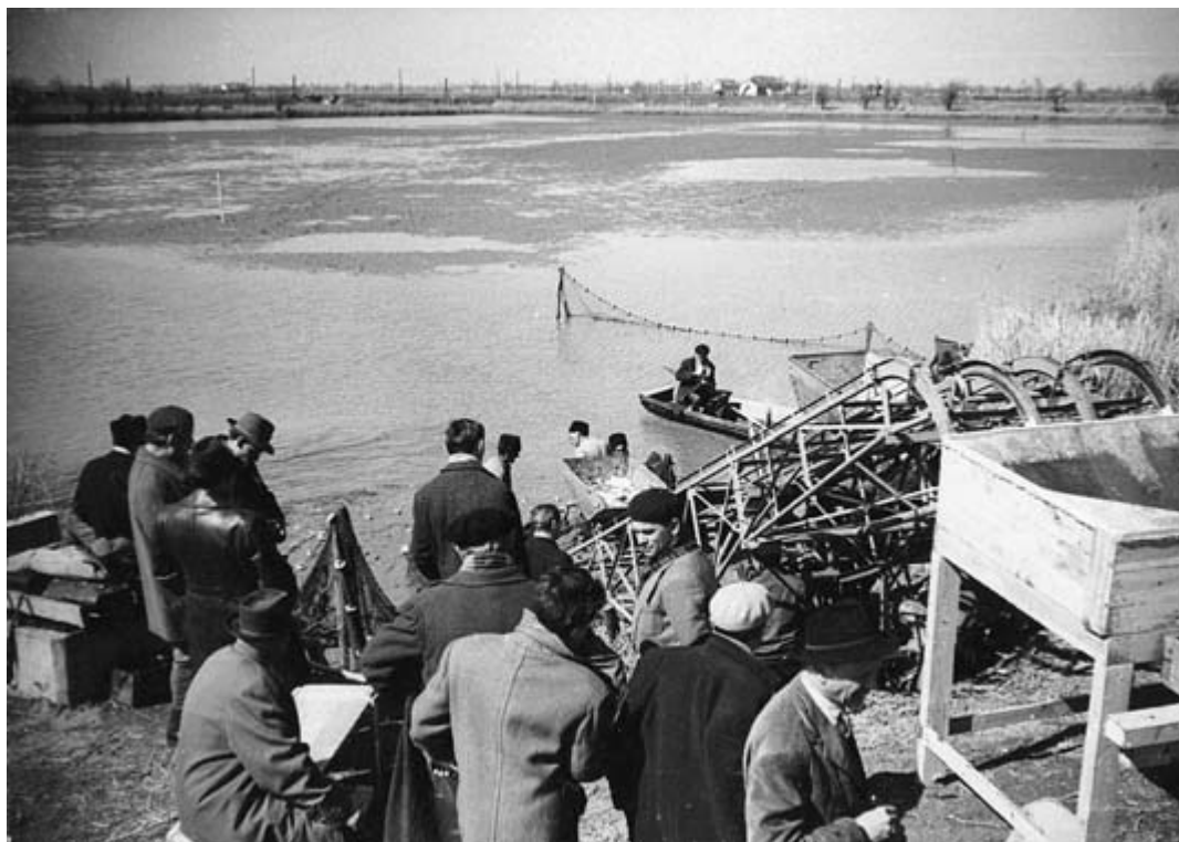
Fig. 11.5 Conveyor belts for lifting fish, used in Hungary. (Courtesy of Josef Kovari.)
