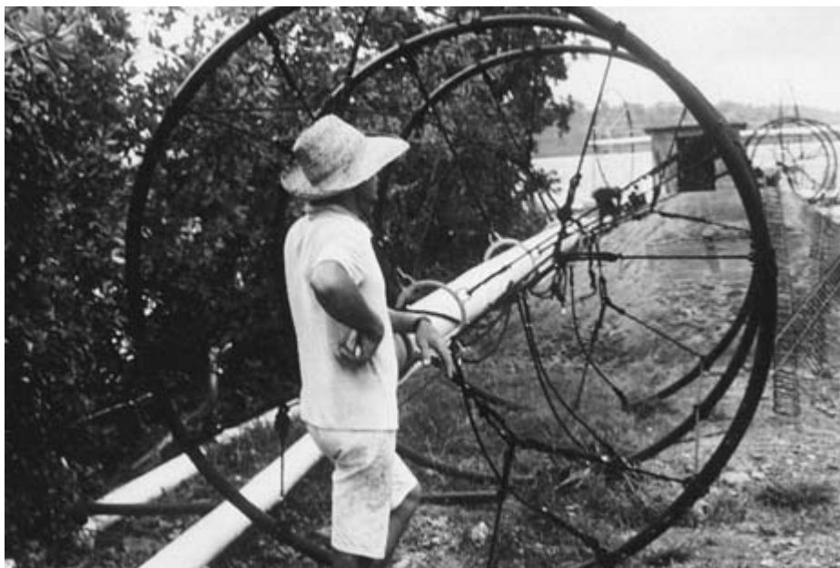
Fig. 6.30 Framework of a collapsible net cage. Note the PVC rings and the central beam.
