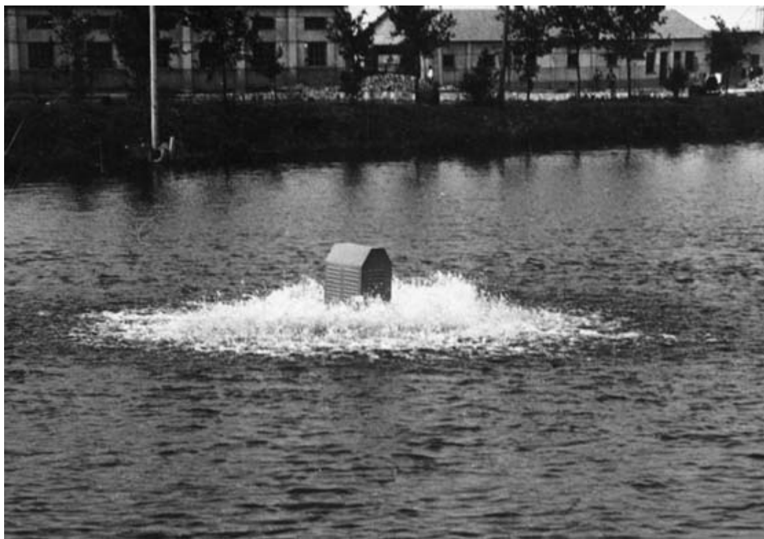
Fig. 16.22 A type of aerator commonly used in Chinese ponds.
