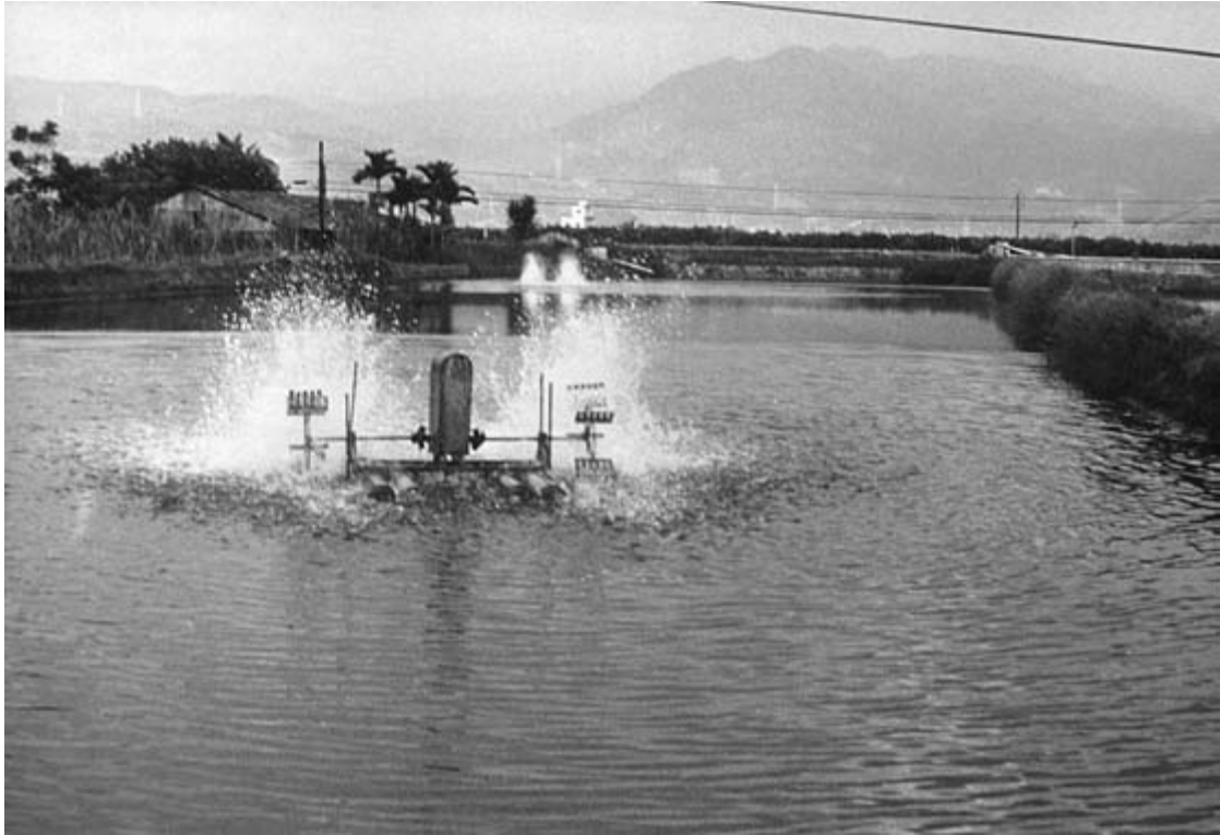
Fig. 25.14 Paddle-wheels used for aeration in intensive pond culture of shrimps in Taiwan. (Courtesy of M. New.)
